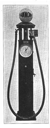
The Board of Trade have examined and tested, with reference to the material of which and the principle on which it is constructed, a pattern of a flow meter of the form shown herein, which has been submitted to the Department under the provisions of Section 6 of the above Act, and have issued a Certificate No. 501 dated 14th March, 1930, that the pattern is not such as to facilitate the perpetration of fraud when used for the measurement of petrol and other liquids of low viscosity.
