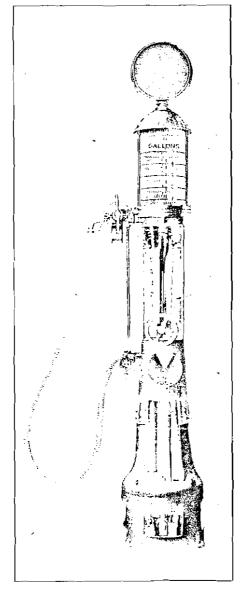
The Board of Trade have examined and tested, with reference to the material of which, and the principle on which it is constructed, a pattern of a liquid measuring and delivering apparatus of the visible container type of 5 gallons Capacity, of the form shown herein, which has been submitted to the Department under the provisions of Section 6 of the above Act, but as the result of the examination was not satisfactory the Board have declined to grant a Certificate of Approval.
